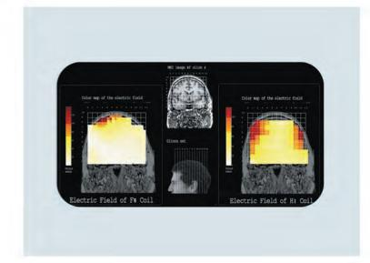
The H1-coil induces fields at depth of 1.8cm, compared to 0.7cm for the figure-8-coil based on measurements in a physiological head model (red indicated the limit of the effective electric field). Source: Rosenberg O, et al. Deep TMS in a resistant major depressive disorder: a brief report. Depress Anxiety. 27:465-9 (2010).
